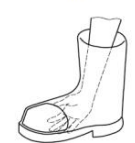
f) Destruction of lining; sharp edges
