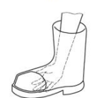
f) Destruction of lining; sharp edges
