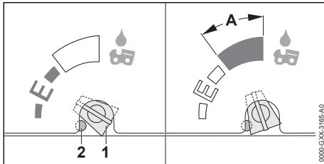
The oil feed rate is suitable for most applications when the oil pump adjusting screw (1) is in position E (Ematic).
