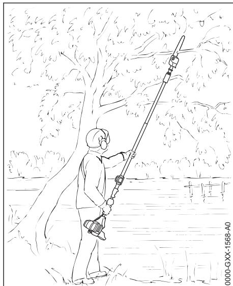
The machine's long reach makes it possible to prune branches that are overhanging obstacles, such as rivers or lakes. The tool angle in this case depends on the position of the branch.
