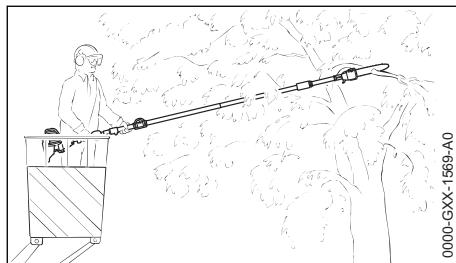
The machine's long reach enables cutting to be performed next to the trunk without the risk of the lift bucket damaging other branches. The tool angle in this case depends on the position of the branch.
