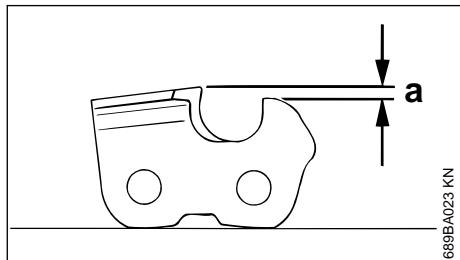
The depth gauge determines the height at which the cutter enters the wood and thus the thickness of the chip removed.
