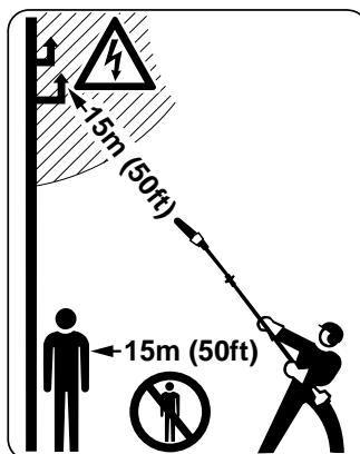
Do not allow other persons within a radius of 15 m of your own position due to falling branches and ejected wood particles – **Risk of injury!**
