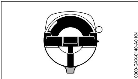
Then the markings on fuel cap and oil tank will align
