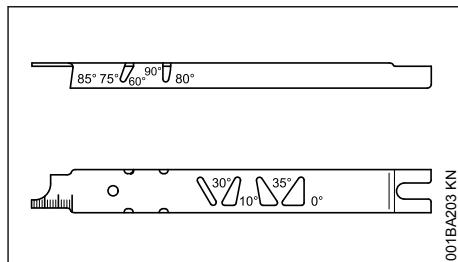
Use a STIHL filing gauge (special accessory, see table "Sharpening Tools"). This is a universal tool for checking the filing and side plate angles, depth gauge setting, cutter length and groove depth. It also cleans the guide bar groove and oil inlet holes.
