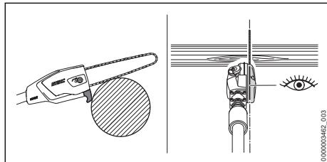
To avoid pinching the saw, position the bar in the area of the housing against the branch and then perform the cross-cut from the top downward. The saw chain can be positioned precisely using the gauge bar.
