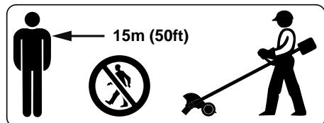
There is a risk of accident from ejected objects within a wide area around the working space, so you must ensure that there is no-one within a 15 m radius of the machine. This distance must also be maintained in relation to objects (vehicles, window panes) – **risk of property damage!** Even at distances beyond 15 m, the danger cannot be ruled out.
