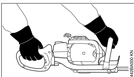
Right hand on the control handle and left hand on the handlebar.
