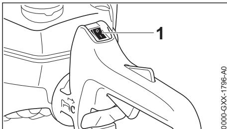
The stop switch (1) is in the normal run position I.
