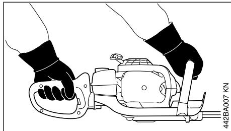
Left hand on the control handle and right hand on the handlebar.
