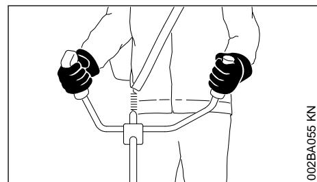
Right hand on control handle, left hand on grip on handlebar.
