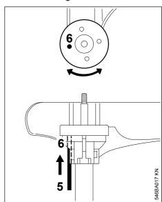
► To block the shaft, insert a suitable tool (5) through the holes (6) in the deflector and thrust plate – turn the thrust plate back and forth if necessary.
