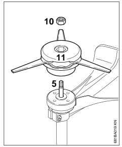
► Push thrust plate onto the shaft
