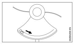
An arrow shows the direction of rotation of the cutting attachments.
