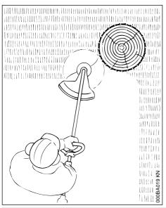
Nylon line achieves a soft cut for edging and trimming around fence posts, trees, etc. – less risk of damaging tree bark.
