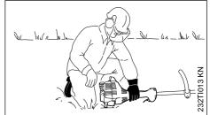
Place the unit on the ground: It must rest securely on the engine support and the deflector.
