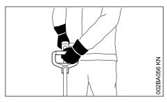
Left hand on the loop handle, right hand on the shaft handle, even if you are left-handed.
