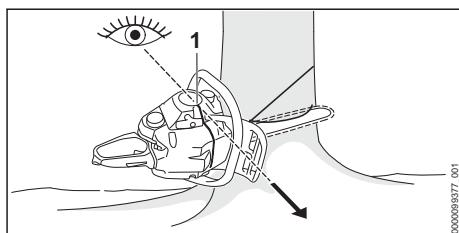
When making the notch, use the gunning sight (1) on the saw to check the desired direction of fall:
