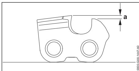
The depth gauge determines the depth to which the cutter penetrates the wood and thus the chip thickness.
