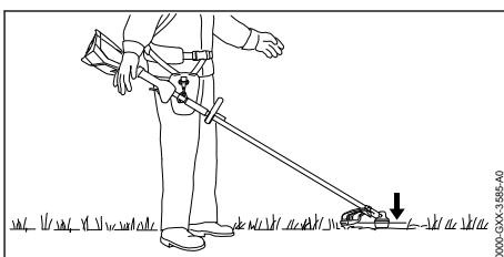
The metal cutting attachment must hover at a height of about 8 in. (20 cm) above the ground should come to rest gently on the ground.
