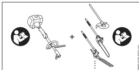
In the STIHL KombiSystem, a KombiEngine (gas-powered) or KombiMotor (battery-powered) can be combined with an assortment of KombiTools to produce different power tools.
