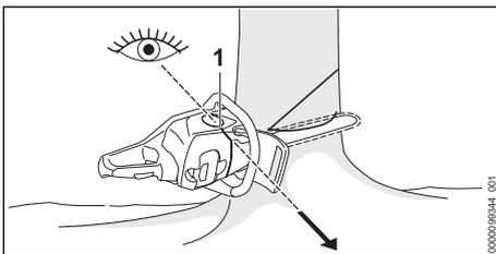
When making the notch, use the gunning sight (1) on the saw to check the desired direction of fall:
