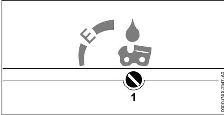
The chain oil feed rate is suitable for most applications when the oil flow adjusting screw (1) is in position **E** (Ematic).
