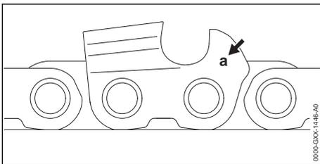
The chain pitch marking (a) is embossed in the area of the depth gauge of each cutter.
