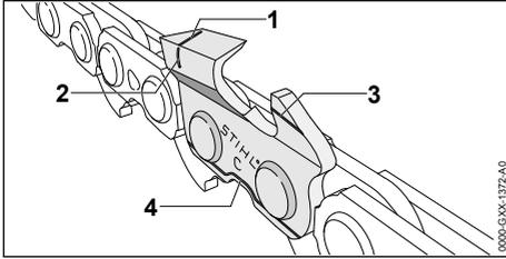
STIHL chain is manufactured with wear marks to help the operator identify excessive wear. The wear marks depicted above (1 - 4) must remain visible.
